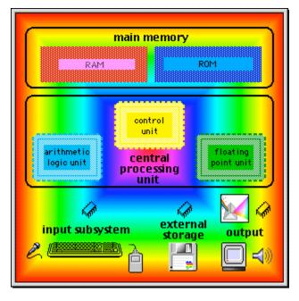
A slightly less crude oversimplification divides a computer into five elements: arithmetic and logic subsystem, control subsystem, main storage, input subsystem, and output subsystem.
